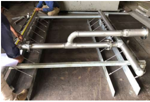
Sand Jetting OR Fluidising System
