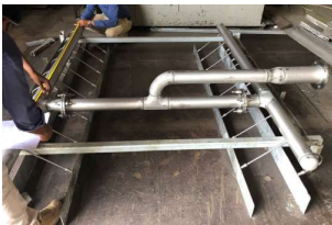
Sand Jetting OR Fluidising System
